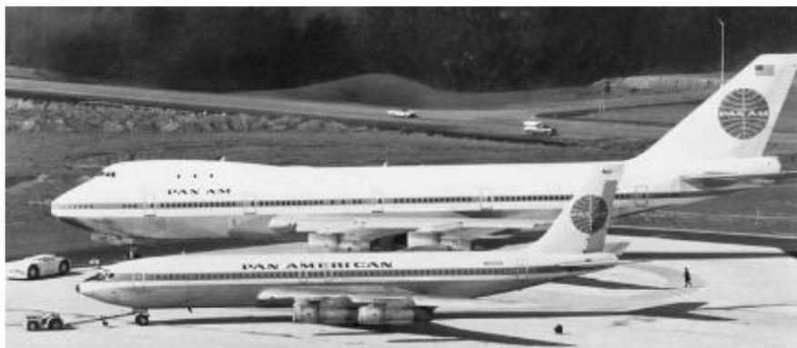
The pilot's eye level when sitting on a 747 flight deck is exactly **32 feet above ground (9,76 metres)**, regardless of their physical size. There is a marker on the side of the cockpit just within the pilot's peripheral vision. The pilot adjusts the seat so that his eye is at the level of the marker.
